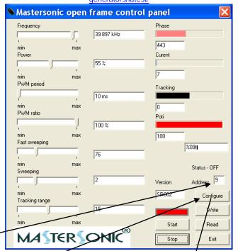
This address is related to the label placed on the generator (here 9). Write the number you see on the generator.
